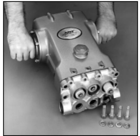
Rotate Crankshaft to position plungers
