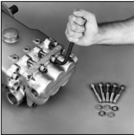
Removal of Discharge Socket Head Screws
