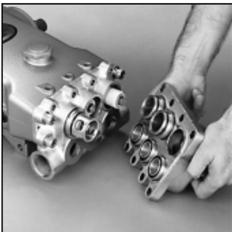
Removal of Discharge Valve Spacers
