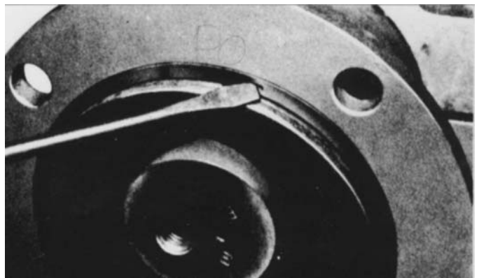
Figure 4.3. Typical Retaining Ring Removal
