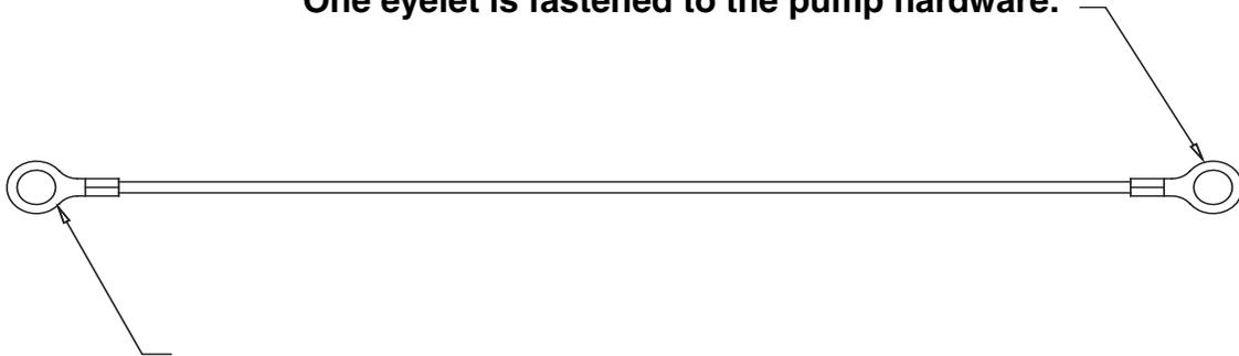
One eyelet is installed to a true earth ground.
