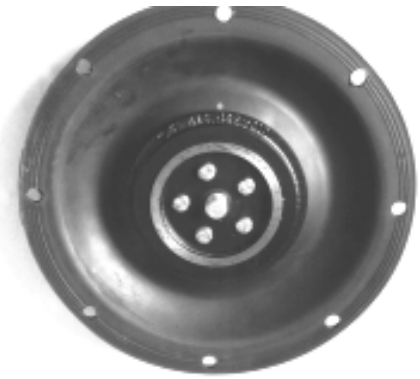
Figure 6: Align hexhead capscrews and tighten
