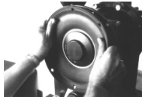
Figure 7: Align diaphragm holes with chamber holes
